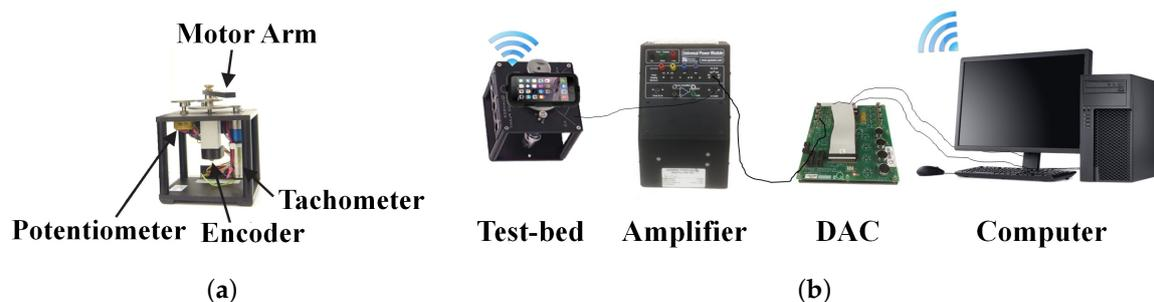
**Figure 1.** (a) DC motor test-bed and (b) experimental setup with a PC-based DAC.
