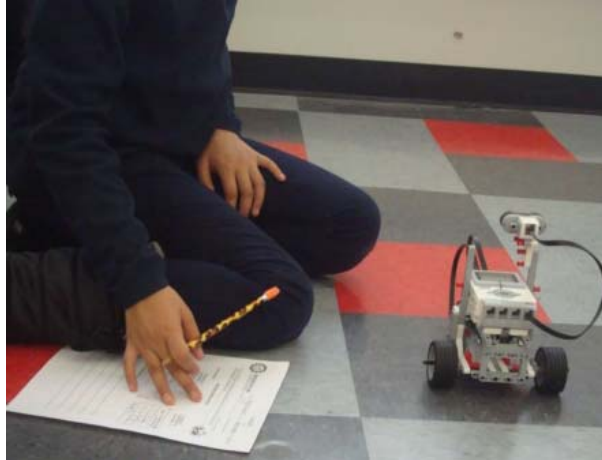
Figure 2: A student observes the distance travelled by the base robot for different gear ratios and writes the observations on the activity sheet. The student also compares the measurements of the travelled distance using a measurement tape and an ultrasonic sensor attached to the base robot.
